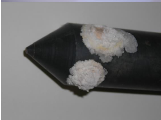
Figure 10: A salt crust on the electrode
