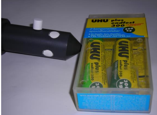
Figure 9: Repair of the ceramic inlet
