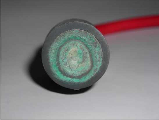
Figure 3: Broken sealing of the Ag/AgCl half-cell causes corrosion of the lead wire. This Ag/AgCl half-cell is permanently damaged.
