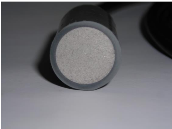
Figure 1: A proper outer surface of the Ag/AgCl half-cell.
